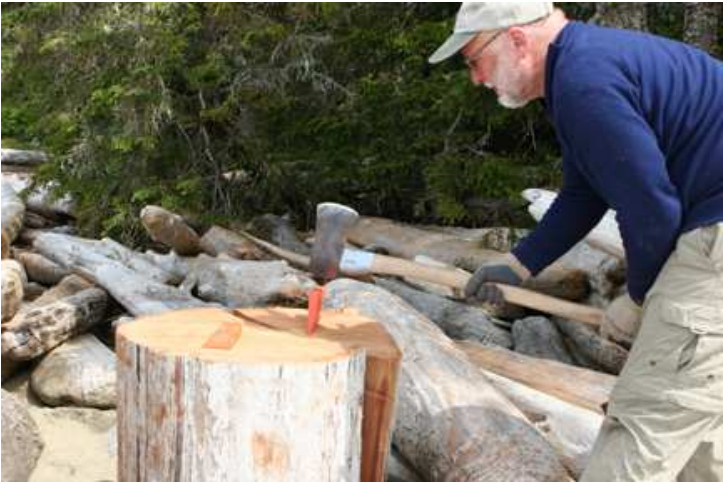
Sawing out and splitting shakes on the beach. Thanks to Ed and Sue Putnam for these photos.
